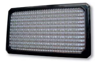
The highly efficient worklight with 60 LEDs and flat design has a power consumption of only 11 Watt. To achieve the same output with a halogen light, 70 Watt (e.g. H3) are required.
