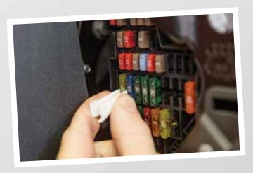
Remove the fuse for the "Horn" circuit from the fuse box in order to cut the power supply of the acoustic signaling units for the duration of the electric connection.
